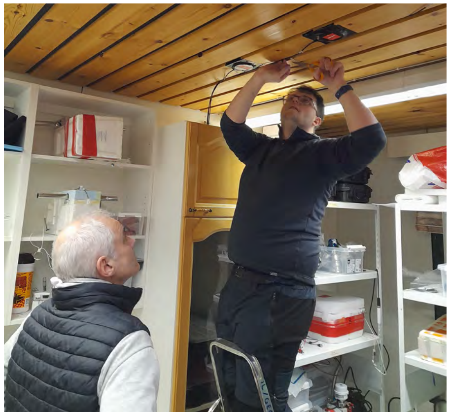
Right: Rich Fitton (l) and Grant Henshaw (r) installing heat flux sensors on the ceiling of a building.
