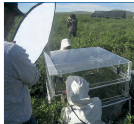
During sunny conditions, a diffuser screen (translucent panel, left) was used to manipulate the light climate, removing direct irradiance from the shrub canopy within the Perspex chamber (centre) to generate a diffuse light environment. During cloudy conditions, opaque white panels were used similarly to enhance illumination of the chamber by concentrating reflected diffuse light.
